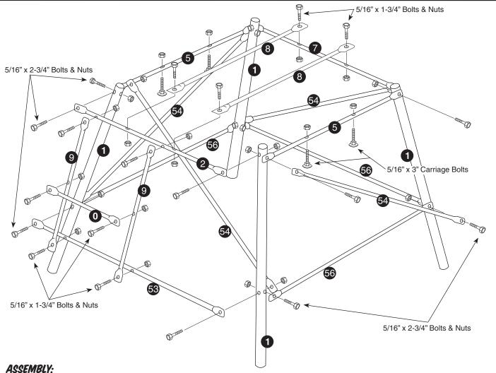
Assemble Front Side – Use lower set of leg holes.
